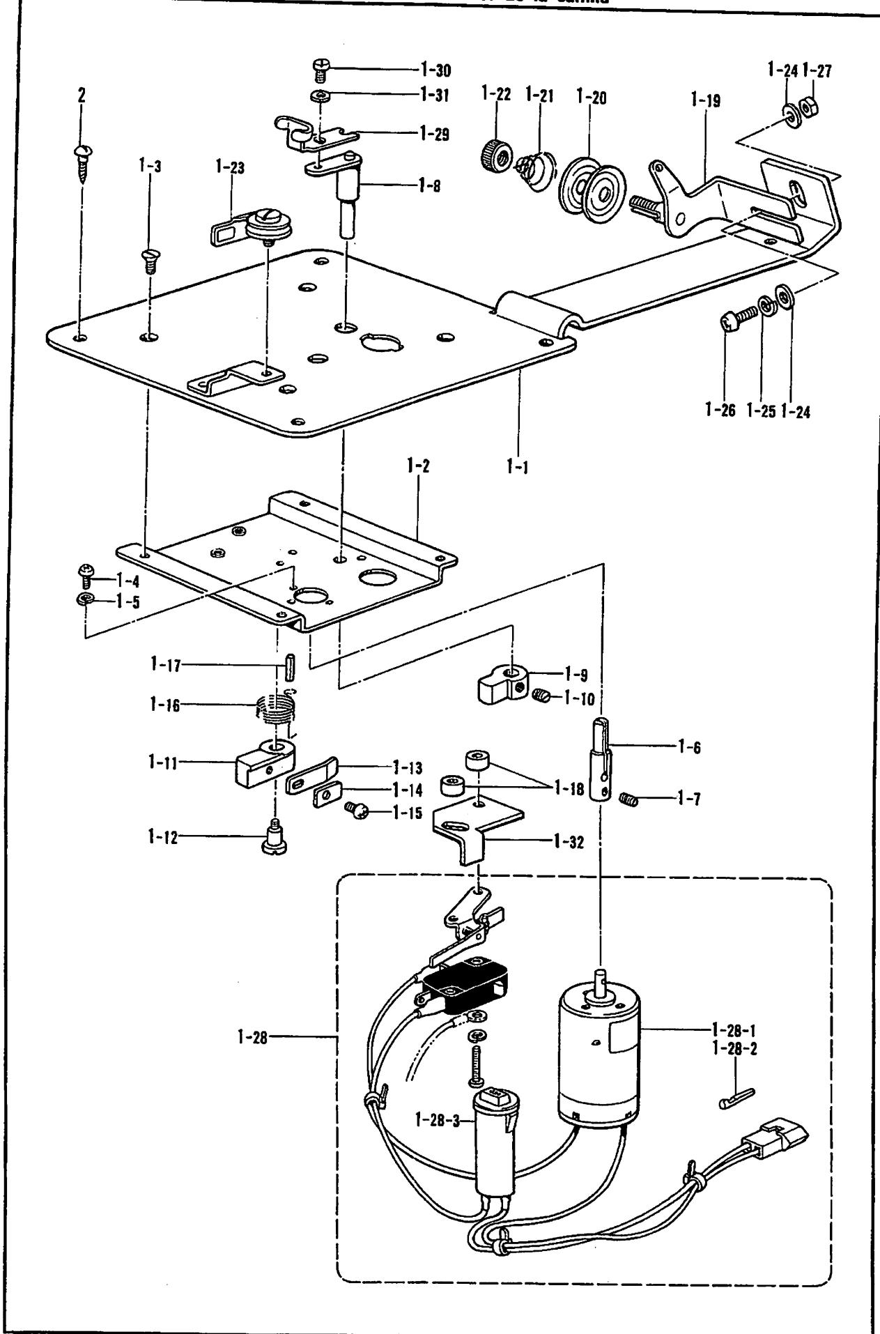
M. 糸巻関係/Bobbin winder mechanism/Spuler/
