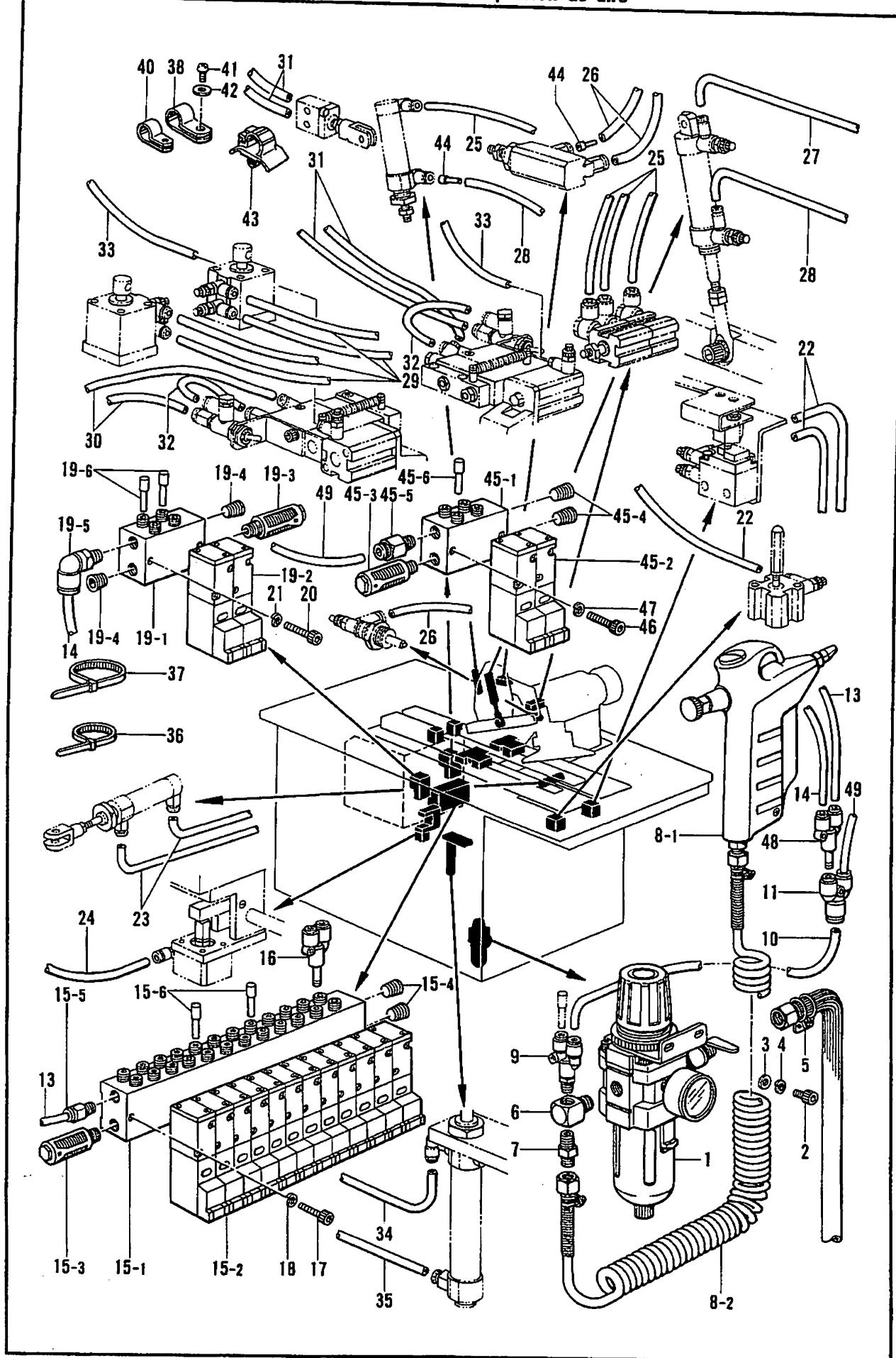
R. 空圧関係/Air pressure mechanism/Luftdruck/
