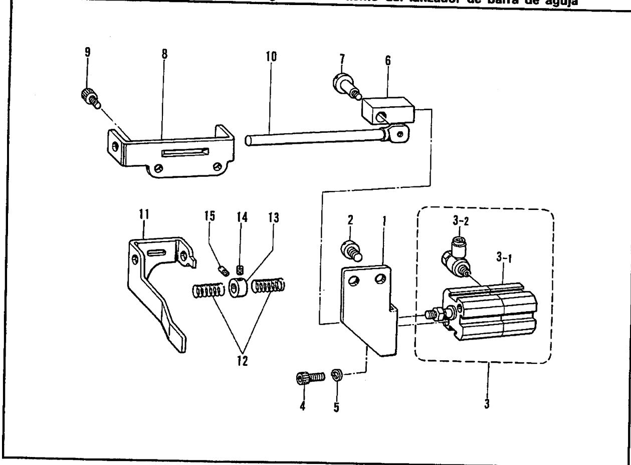
E. 下軸関係/Lower shaft mechanism/Untere Welle/
