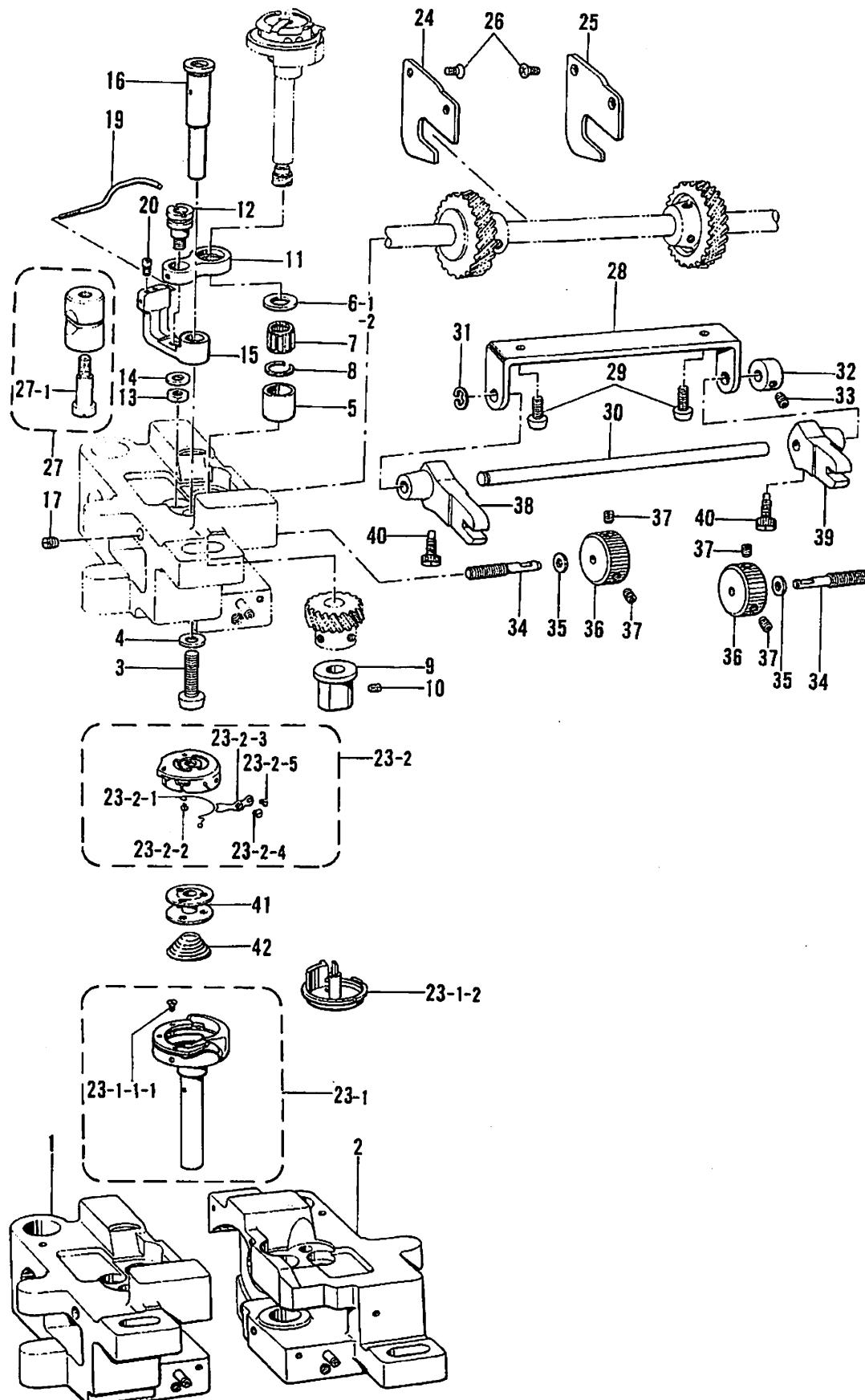
G. カマ関係/Rotary hook mechanism/Greifervorrichtung/
